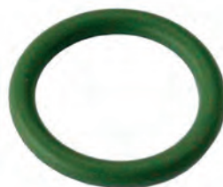
250445# O-ring Replacing: -014.3MG Thickness 2.30 mm, ID 14.30 mm, Colour Green, Material HNBR
