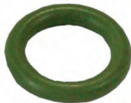
250444 O-ring Replacing: -008MG Servicing: 8600889, 8FK351316-141 Thickness 2.00 mm, ID 8.00 mm, OD 12.00 mm, Colour Green, Material HNBR
