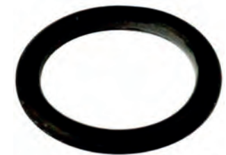
250500# O-ring Replacing: -014.6MN Thickness 2.40 mm, ID 14.60 mm, Colour Black, Material Nioprene
