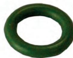
252165# O-ring Replacing: -108G Thickness 2.62 mm, ID 6.02 mm, OD 11.00 mm, Colour Green, Material HNBR
