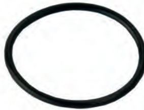
250604# O-ring Replacing: -126MN Thickness 2.00 mm, ID 29.50 mm, Colour Black, Material Nioprene
