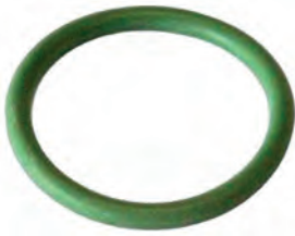
250503 O-ring Replacing: -014X1.5MG Thickness 1.50 mm, ID 14.00 mm, Colour Green, Material HNBR
