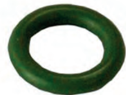
250452# O-ring Replacing: -101G Thickness 1.78 mm, ID 6.07 mm, Colour Green, Material HNBR
