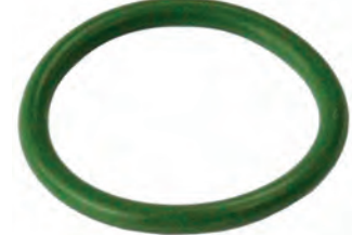
250499# O-ring Thickness 2.40 mm, ID 21.60 mm, Colour Green, Material HNBR
