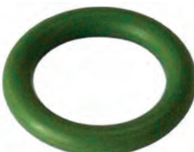
250507 O-ring Servicing: 90457635 Thickness 2.00 mm, ID 9.00 mm, Colour Green, Material HNBR
