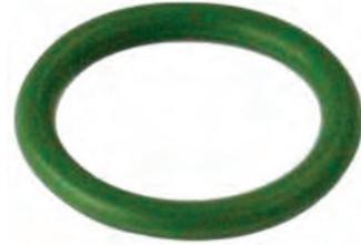
250496# O-ring Replacing: -515DG Thickness 1.88 mm, ID 12.01 mm, Colour Green, Material HNBR
