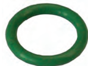
250453 O-ring Replacing: -012G Servicing: 10517C, 44720-09897, 699298, 8FK351316-141, 90457635, HFC134A Thickness 1.78 mm, ID 9.25 mm, Colour Green, Material HNBR
