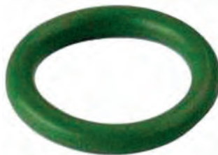
250493# O-ring Replacing: -955MDG Thickness 1.88 mm, ID 9.60 mm, Colour Green, Material HNBR
