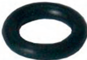
251598# O-ring Replacing: -006MN Servicing: 0001416062, 0001416067, 11.139.025, 19024049, AZK5184, IM562 Thickness 2.00 mm, ID 6.00 mm, Colour Black, Material Nioprene
