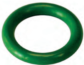
250490# O-ring Replacing: -208G Thickness 3.53 mm, ID 15.47 mm, Colour Green, Material HNBR
