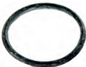
252600# O-ring Replacing: -028MN Thickness 2.50 mm, ID 28.00 mm, Colour Black, Material Rubber
