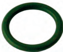
250441 O-ring Replacing: -013G Thickness 1.78 mm, ID 10.82 mm, Colour Green, Material HNBR
