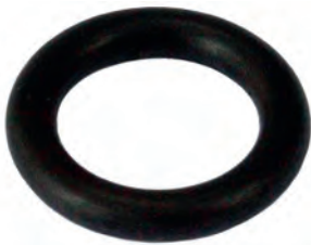
250488# O-ring Replacing: -207N Thickness 3.53 mm, ID 13.87 mm, Colour Black, Material Nioprene
