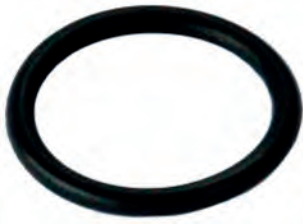
250190# O-ring Replacing: -015N Thickness 1.78 mm, ID 14.00 mm, Colour Black, Material Niopprene
