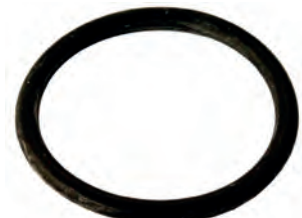
250731# O-ring Replacing: -026MN Servicing: 8FK351316-141 Thickness 2.50 mm, ID 26.00 mm, OD 30.50 mm, Colour Black
