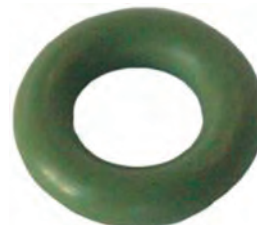
252583# O-ring Replacing: -007G Thickness 1.78 mm, ID 3.69 mm, Colour Green, Material HNBR
