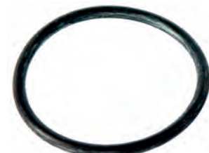
252652# O-ring Replacing: -126N Thickness 2.62 mm, ID 34.60 mm, Colour Black, Material Rubber
