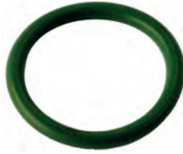
250442 O-ring Replacing: -015G Thickness 1.78 mm, ID 14.00 mm, Colour Green, Material HNBR
