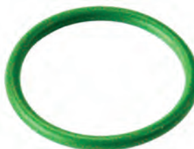
250672 O-ring Replacing: -018G Thickness 1.78 mm, ID 18.77 mm, Colour Green, Material HNBR
