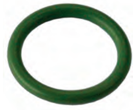
250447 O-ring Replacing: -016.5X2.43MG Thickness 2.43 mm, ID 16.50 mm, Colour Green, Material HNBR
