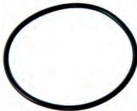
252632# O-ring Replacing: -048N Thickness 2.00 mm, ID 48.00 mm, Colour Black, Material Rubber
