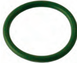
250443 O-ring Replacing: -017G Servicing: 228000-7710, NAD100952 Thickness 1.78 mm, ID 17.17 mm, Colour Green, Material Rubber
