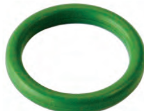
250642# O-ring Replacing: -116RG Thickness 3.65 mm, Height 2.79, ID 18.89 mm, Colour Green, Material HNBR
