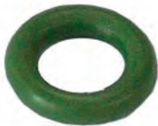
250439# O-ring Replacing: -008G Thickness 1.78 mm, ID 4.47 mm, Colour Green, Material HNBR
