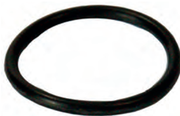
251425# O-ring Replacing: -121N Thickness 2.62 mm, ID 26.65 mm, Colour Black, Material Nioprene
