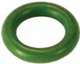
250487# O-ring Replacing: 92470-N8210 Thickness 1.77 mm, ID 6.88 mm, Colour Green, Material HNBR
