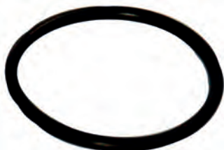
251257# O-ring Replacing: -021N Thickness 1.78 mm, ID 23.52 mm, Colour Black, Material Nioprene
