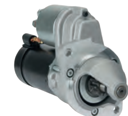
110856 Starter 12 V, 0.6 kW Replacing: AZE0303, 11.130.134, 11.130.034 Servicing: Renault B+ M8, Length 208.50, Drive type Steel, Gear type DD/GR, Clutch type Dry, Mount. holes 2 (0) A: 66.00 B: 21.00 mm
