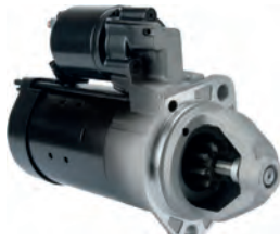
113181 Starter 12 V, 2.3 kW Replacing: 0001223021, 0001223016 Servicing: Bomag, JCB, KHD B+ M8, Length 258.00, Drive type Steel, Gear type GR, Mount. holes 2 (0) A: 82.50 B: 23.00 mm
