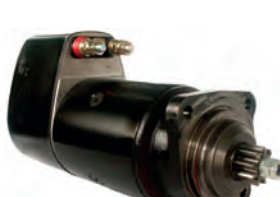
111218 Starter 24 V, 5.4 kW Replacing: R23.33, 6330000 Servicing: Volvo Penta B+ M10, B- M10, Length 388.00, Drive type Steel, Gear type DD, Mount. holes 3 (0), Insulated return A: 89.00 B: 48.00 mm
