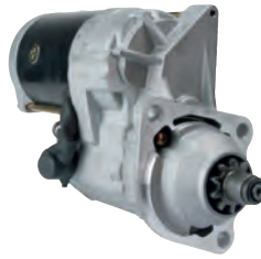
114449 Starter 12 V, 4.0 kW Replacing: 228000-6872, 228000-6871, 228000-6870 Servicing: Case B+ M10, Length 318.00, Drive type Steel, Gear type GR, Mount. holes 3 (0) A: 89.00 B: 47.50 mm
