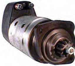
110205 Starter 24 V, 6.5 kW Replacing: R22.22, 0220000 Servicing: Volvo B+ M10, Length 407.00, Drive type Steel, Gear type DD, Mount. holes 3 (0), Waterproof A: 89.00 B: 47.50 mm
