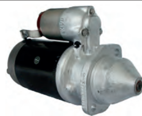
111001 Starter 12 V, 3.0 kW Replacing: AZJ3557, AZJ3320, AZF4220, 11.131.829, 11.130.898, 11.130.254 Servicing: Lamborghini, Same, Steyr B+ M10, Length 340.00, Drive type Steel, Gear type DD, Mount. holes 2 (0) A: 82.00 B: 21.60 mm
