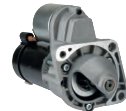
111025 Starter 12 V, 0.8 kW Replacing: R80K, R80.04 Servicing: Autobianchi, Fiat, Lancia B+ M8, Length 209.00, Drive type Steel, Gear type DD/GR, Mount. holes 3 (2) A: 64.00 B: 11.00 mm
