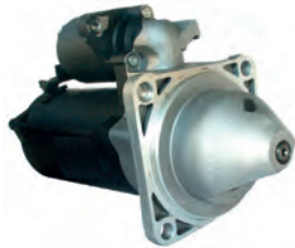
113183 Starter 24 V, 4.0 kW Manufacturer: Bosch Replacing: 0001231010 Servicing: Iveco B+ M10, Length 315.00, Drive type Steel, Gear type GR, Clutch type Dry, Mount. holes 3 (0) Alternative no.: 116347 A: 110.00 B: 28.00 mm
