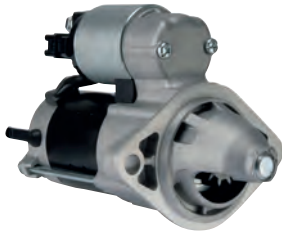
114419 Starter 12 V, 1.2 kW Replacing: 428000-0341, 428000-0340 Servicing: Pontiac, Toyota B+ M8, Length 194.00, Drive type Steel, Mount. holes 2 (0) A: 74.00 B: 14.80 mm
