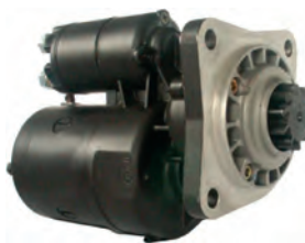
113269 Starter 12 V, 3.0 kW Manufacturer: Magneton Replacing: 0001359094 Servicing: Atlas Copco, Barber Greene, Benford, Case, Daewoo, Matbro, Perkins, Thwaites B+ M10, Length 234.50, Drive type Steel, Gear type GR, Mount. holes 3 (0) A: 88.80 B: 31.50 mm
