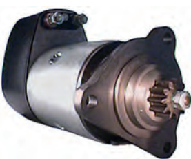
110582 Starter 24 V, 5.4 kW Replacing: R23.06, 6060000 Servicing: Iveco B+ M10, B- M10, Length 384.00, Drive type Steel, Gear type DD, Mount. holes 3 (0) A: 92.00 B: 47.00 mm
