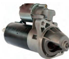
110847 Starter 12 V, 1.4 kW Replacing: AZE2525, 11.130.651 Servicing: Opel, Saab, Toyota, Vauxhall B+ M8, Length 242.50, Drive type Steel, Gear type GR, Mount. holes 2 (1) A: 82.50 B: 19.00 mm
