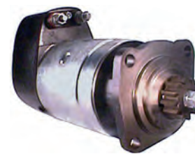
111231 Starter 24 V, 6.6 kW Replacing: R22.38, 0380000 Servicing: Renault V.I. B+ M10, B- M10, Length 405.00, Drive type Steel, Gear type DD, Mount. holes 3 (0), Insulated return A: 89.00 B: 40.25 mm
