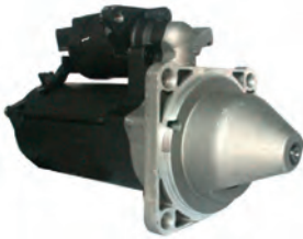
113182 Starter 12 V, 3.0 kW Replacing: 0001262008, 0001262007, 0001230023, 0001230010, 0001230007 Servicing: New Holland B+ M10, Length 320.00, Drive type Steel, Gear type GR, Mount. holes 3 (0) A: 110.00 B: 27.00 mm
