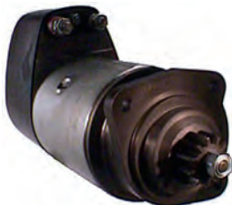
110207 Starter 24 V, 5.4 kW Replacing: R23.10, 6100000 Servicing: Volvo, Volvo BM B+ M10, B- M10, Length 387.00, Drive type Steel, Gear type DD, Mount. holes 3 (0) A: 89.00 B: 47.00 mm
