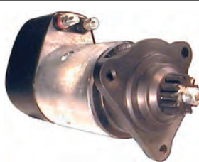
110980 Starter 24 V, 5.4 kW Replacing: R23.34, 6340000 Servicing: Volvo B+ M10, B- M10, Length 387.00, Drive type Steel, Gear type DD, Mount. holes 3 (0) A: 92.00 B: 47.00 mm
