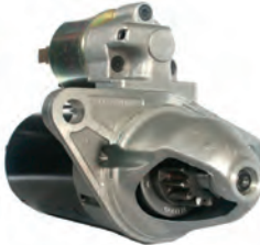
113281 Starter 12 V, 1.1 kW Replacing: 0001107080 Servicing: MG, Rover B+ M8, Length 231.40, Drive type Steel, Gear type GR, Clutch type Dry, Mount. holes 2 (0) A: 75.00 B: 43.00 mm
