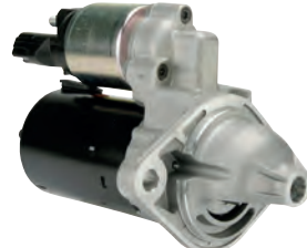
113271 Starter 12 V, 1.1 kW Replacing: 0001107434, 0001107433, 0001107088 Servicing: Toyota B+ M8, Length 204.00, Drive type Steel, Gear type GR, Clutch type Dry, Mount. holes 2 (1) A: 73.90 B: 15.00 mm
