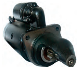
113184 Starter 24 V, 4.0 kW Manufacturer: Bosch Replacing: 0001368069 Servicing: Case B+ M10, Length 340.00, Drive type Steel, Gear type DD, Mount. holes 3 (0) A: 88.70 B: 48.00 mm
