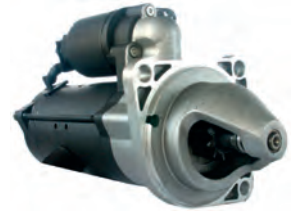
113277 Starter 24 V, 4.0 kW Replacing: 0001231011 Servicing: Iveco B+ M10, Length 315.00, Drive type Steel, Gear type GR, Mount. holes 3 (0) A: 109.80 B: 27.50 mm
