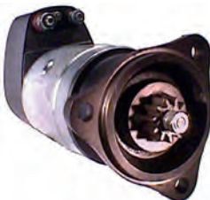
110213 Starter 24 V, 6.6 kW Replacing: R22.07, 0070000 Servicing: Fiat, Iveco B+ M12, B- M10, Length 407.00, Drive type Steel, Gear type DD, Mount. holes 3 (0) A: 115.00 B: 20.80 mm
