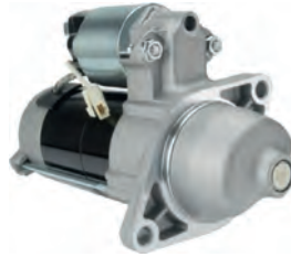
114485 Starter 12 V, 1.1 kW Replacing: 228000-7091, 228000-7090, 228000-5401, 228000-5400 Servicing: Bobcat, Kubota B+ M8, Length 211.00, Drive type Steel, Gear type GR, Mount. holes 2 (0) A: 66.00 B: 18.00 mm
