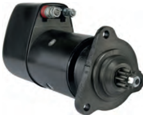
110206 Starter 24 V, 5.4 kW Replacing: R23.08, 6080000 Servicing: Claas, Fiat-Allis, Kässbohrer, MAN, Mercedes-Benz, Neoplan, Setra B+ M12, B- M10, Length 390.00, Drive type Steel, Gear type DD, Mount. holes 3 (0) A: 92.00 B: 47.50 mm
