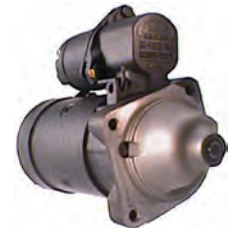
110338 Starter 12 V, 0.8 kW Replacing: R80Z Servicing: Fiat, Lancia, Zastava B+ M8, Length 254.00, Drive type Steel, Gear type DD, Mount. holes 3 (3) A: 66.90 B: 12.00 mm
