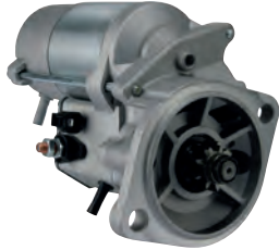
114429 Starter 12 V, 2.0 kW Replacing: 228000-8890 Servicing: Isuzu B+ M8, Length 218.00, Drive type Steel, Gear type GR, Mount. holes 2 (0) A: 95.00 B: 10.00 mm
