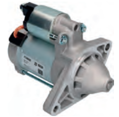
114660 Starter 12 V, 1.2 kW Replacing: 428000-4550, 428000-3372, 428000-3371, 428000-3370 Servicing: Toyota B+ M8, Length 189.00, Gear type GR, Mount. holes 2 (1) A: 74.00 B: 11.50 mm
