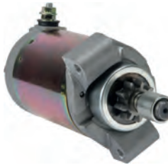
114486 Starter 12 V Replacing: 128000-2760 Servicing: John Deere, Kawasaki B+ M6, Length 173.00, Drive type Steel, Gear type DD, Mount. holes 2 (0) B: 20.00 mm
