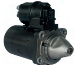
110365 Starter 12 V, 0.8 kW Replacing: R80.02, E80C, 8100000, 8020020000 Servicing: Autobianchi, Fiat, Lancia, Seat B+ M8, Length 236.50, Drive type Steel, Gear type DD, Mount. holes 3 (3) A: 62.00 B: 12.50 mm
