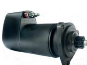
110981 Starter 24 V, 5.4 kW Replacing: AZK5553, AZK5184, 11.139.514, 11.139.025 Servicing: DAF B+ M12, B- M10, Length 387.00, Drive type Steel, Gear type DD, Mount. holes 3 (0) A: 110.00 B: 47.50 mm
