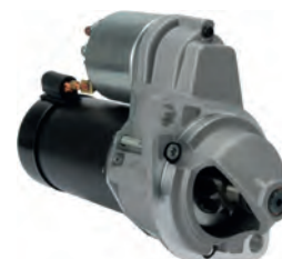
111015 Starter 12 V, 1.1 kW Replacing: AZD2127, 11.131.928 Servicing: Lombardini, Various Agriculture Vehicles B+ M8, Length 216.25, Drive type Steel, Gear type GR, Clutch type Dry, Mount. holes 2 (0) A: 76.20 B: 15.00 mm
