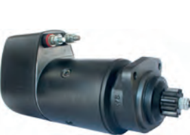
110932 Starter 24 V, 5.4 kW Replacing: R23.24 Servicing: DAF B+ M10, B- M10, Length 384.50, Drive type Steel, Gear type DD, Mount. holes 3 (0), Insulated return A: 88.85 B: 47.00 mm
