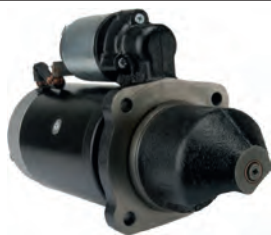
110551 Starter 12 V, 3.0 kW Replacing: R11B, R11.02 Servicing: Lamborghini, Same, Ursus, Zetor B+ M10, Length 326.50, Drive type Steel, Gear type DD, Mount. holes 3 (0) A: 89.00 B: 47.00 mm
