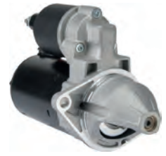
113276 Starter 12 V, 1.1 kW Replacing: 0001107436, 0001107435, 0001107413, 0001107412, 0001107409, 0001107408, 0001107405, 0001107404 Servicing: Chevrolet, Daewoo, Fiat, Mercedes-Benz, Opel, Saab, Vauxhall B+ M8, Length 200.00, Drive type Steel, Gear type GR, Mount. holes 2 (0) A: 67.90 B: 19.00 mm
