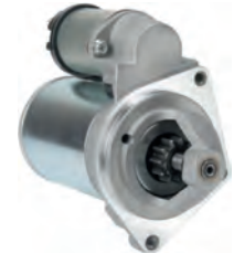
110352 Starter 12 V, 1.3 kW Replacing: R100.3, R100.03, E100L-1.5/12, 803000.2 Servicing: Fiat, Lada B+ M8, Length 201.00, Drive type Steel, Gear type DD, Clutch type Wet, Mount. holes 3 (3) A: 82.50 B: 22.50 mm
