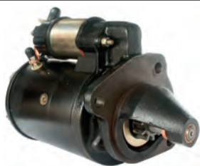
110819 Starter 12 V, 2.8 kW Replacing: AZJ3389, AZJ3206, AZJ3148, 11.131.162, 11.130.632, 11.130.520 Servicing: Eicher, Massey Ferguson, Perkins B+ M8, Length 311.00, Drive type Steel, Gear type DD, Mount. holes 3 (0) A: 92.00 B: 23.00 mm
