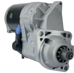
114459 Starter 12 V, 4.8 kW Replacing: 228000-8471, 228000-8470 Servicing: John Deere B+ M12, Length 315.00, Gear type GR, Mount. holes 3 (0) A: 89.00 B: 48.00 mm
