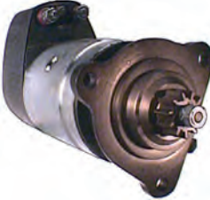
110212 Starter 24 V, 6.6 kW Replacing: R23.26, R22.16, R22.14, 6260000, 0160000, 0140000 Servicing: Iveco, Scania B+ M10, B- M10, Length 407.00, Drive type Steel, Gear type DD, Mount. holes 3 (0) A: 92.00 B: 47.65 mm
